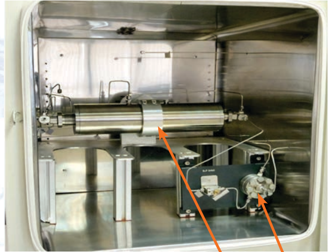
Figure 2. Photo of core flooding system with core holder and U10L
