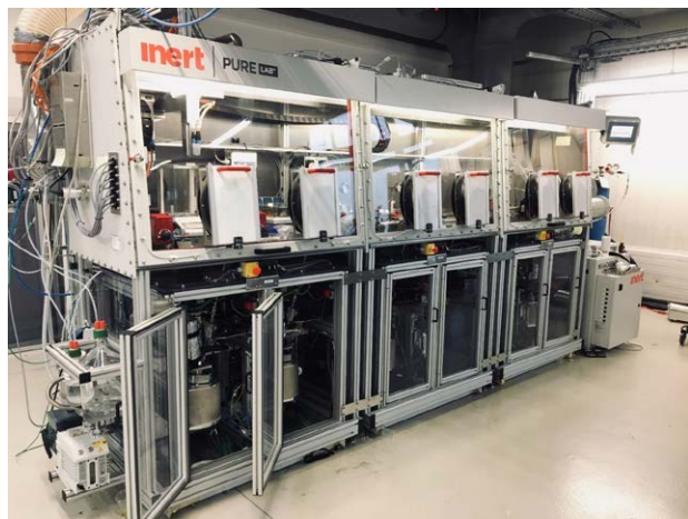
Figure 1: Fully-automated 6 parallel batch polymerization unit
