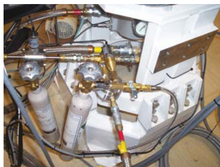
The Equilibar back pressure regulator is shown (center) in front of the helium-cooled cryostat (background).
