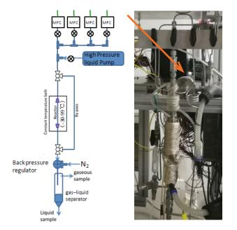
Figure 3: Direct synthesis reactor schematic and photo with an Equilibar LF1 back pressure regulator indicated by arrow.
