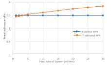
Figure 2: Graph of reactor pressure control at various flow rates with an Equilibar back pressure regulator versus a traditional unit
