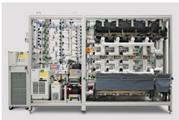
Figure 1: ILS parallel test reactor system for VAM Vinyl-Acetate-Monomer catalyst R&D
