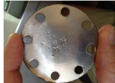
**Figure 5b.** Top view of a SS8 diaphragm used in the Duke SCWO unit. Diaphragm was primarily exposed to air, but also some liquid water. The diaphragm burst after about 5 hours of operation (center indentation is punctured, may not be visible in picture).
