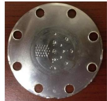
**Figure 5c.** Top and bottom view of a SS8 diaphragm used in the Duke SCWO unit. Diaphragm did not burst, but showed clear signs of wear after only 2 hours of operation with only vapor.
