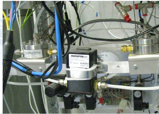
Figure 2: Hydrogen Fuel Cell Experimental Rig (Two Equilibar Back Pressure Regulators piloted by single Proportion Air QPV)
