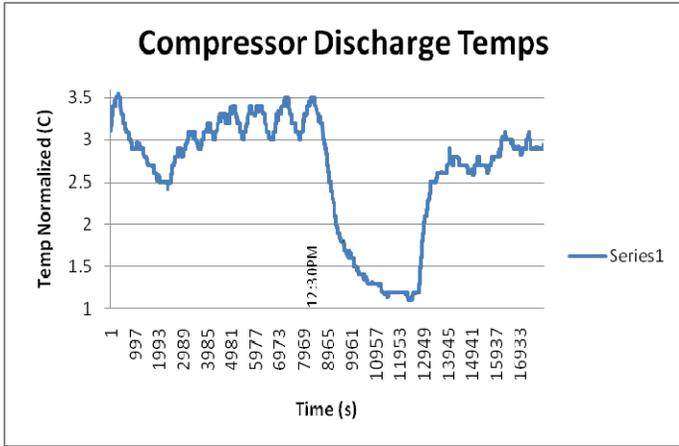
**Fig. 8 Compressor Discharge Line Temperatures Impacted By Room Temperature Variations**
