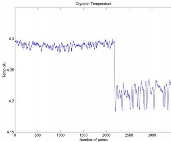
**Fig. 16 Temperature Contrast With BPR Operation**
