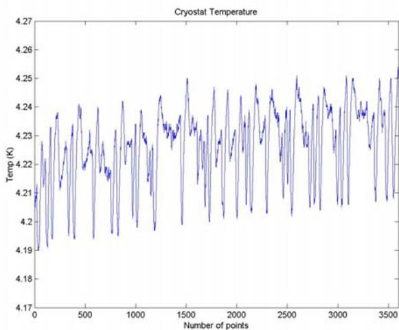
**Fig. 2 Temperature Deviation Before BPR Installation**
