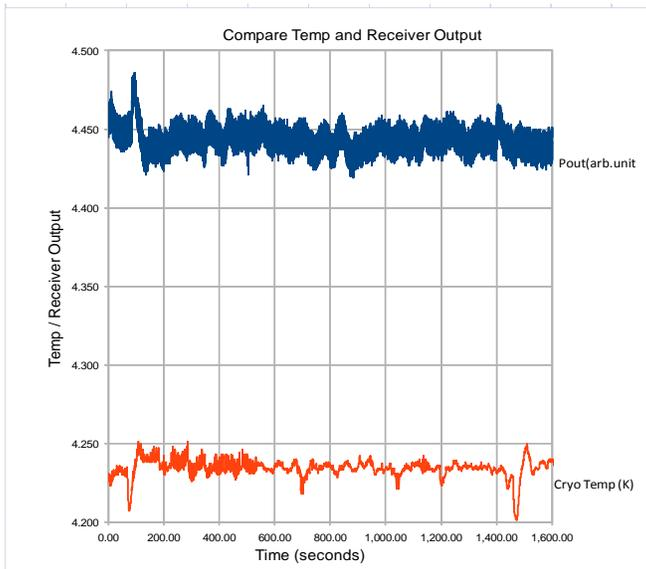
**Fig. 1 Correlation Between Temperature and Power**
