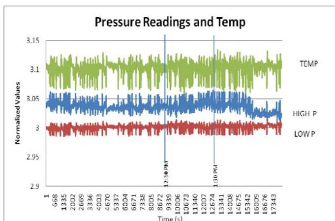
Fig. 6 Cryostat High And Low Pressure Readings
