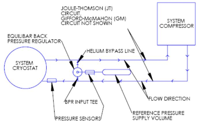
**Fig. 3 Cryostat System Schematic**
