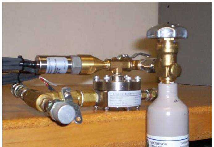
**Fig. 11 BPR Ready For Cryostat Base Installation**
