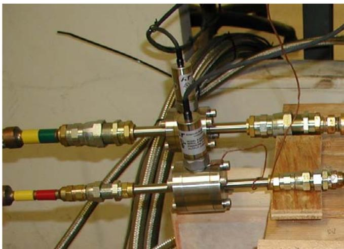
Fig. 5 AST Model 4000 Pressure Sensors
