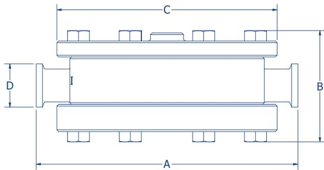
**Fig. 3 FDO Regulator with Active Damping - Dimensional Drawing**
